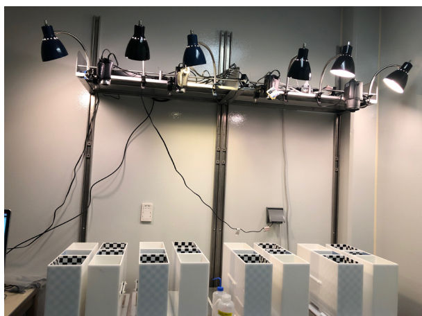
Figure 2. Conditioned place preference room setup with eight apparatus. Each CPP chamber is assigned a box ID (e.g., Box 1). The orientation of each box is antiparallel (rotated 180°) from the adjacent box. The location of each box is permanently fixed. The overhead lights are positioned to avoid shadows on the floor of the compartments. Each camera is positioned to record from two boxes.
