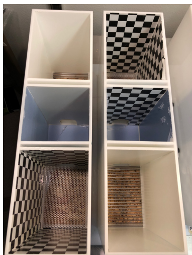
Figure 1. Two conditioned place preference apparatus. The outer compartments (Floor: 12.5 cm x 17 cm; Height: 32.5 cm) are separated by a smaller inner compartment (Floor: 12.5 cm x 11.5 cm; Height: 32.5 cm). The compartment with checkered contact paper has a grid floor with cedar shaving below. The compartment with white contact paper has bar flooring with pine chips below. The middle compartment has a solid gray floor, two gray walls, and two walls with either checkered or white contact paper to match the adjoining outer compartments. Guillotine doors separate the outer compartments from the middle compartment.
