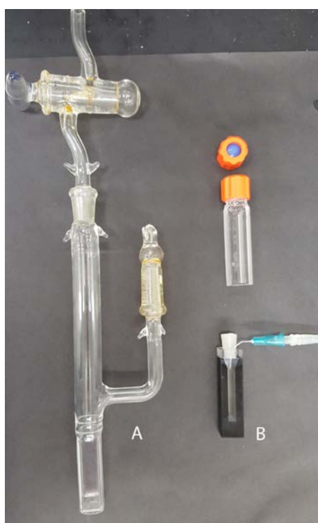
Figure 2. Optical cuvettes that can be used for anaerobic measurements. A. A sealed anaerobic cuvette with a side arm. B. A cuvette with a septum (top) and a standard optical cuvette equipped with a silicone stopper (bottom). Both cuvettes can be used with a gas line to supply argon/nitrogen (shown for the bottom cuvette).
