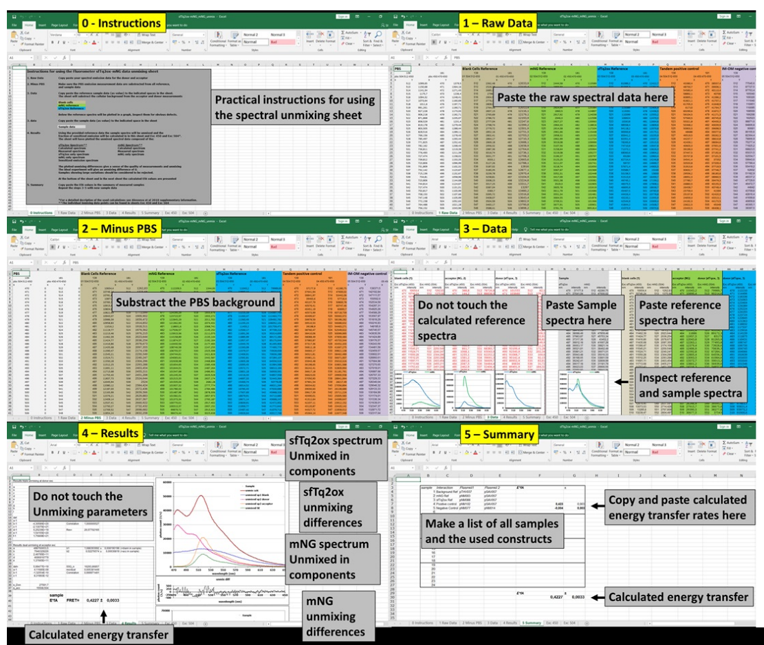
Figure 7. The unmixing process for the calculation of FRET efficiencies as it would appear on the screen. Raw donor and acceptor unmixing calculations that will not be directly used are shown in the high-resolution screenshots in Supplementary file ' Unmixing screens.pptx '.
