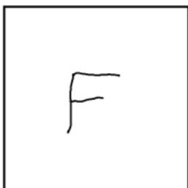
Figure 3. An “F” carved into the center of a 22 x 22 mm ITO coverslip. Note the size of the “F” relative to the size of the coverslip.
