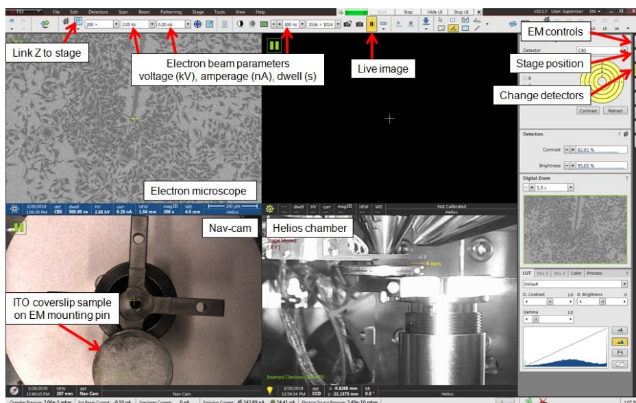
Figure 16. Annotated screen capture of the FEI Helios Nanolab™ xT Microscope Control software (version 10.1.7)
