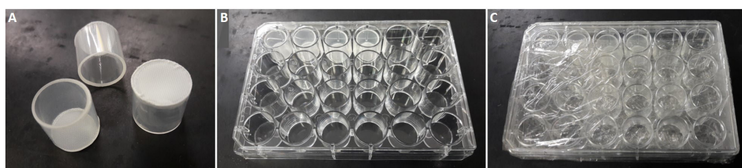
Figure 1. Sample carrier. A. Example of three baskets with mesh-bottom. B. A 24-well plate used for in situ hybridization, with four baskets. C. The same plate, closed and wrapped in plastic film to avoid evaporation during hybridization step.
