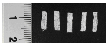
Figure 2. Kimwipe paper strips used to fix sample with the clamps ( ca. 2 mm x 10 mm in length, hand-made)
