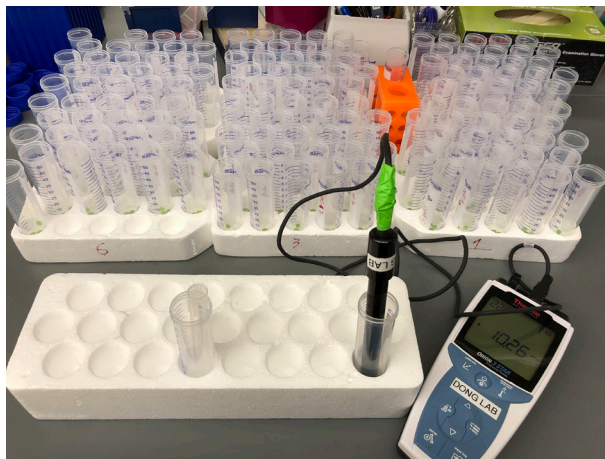
Figure 1. Picture describing ion leakage measurement using the Thermo Scientific Orion Star A322 Electro-conductivity meter
