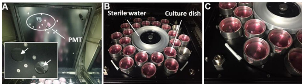
Figure 5. Monitoring bioluminescence in real time. Bioluminescence can be measured in real time using a photomultiplier tube (LM2400) at 35 °C with 5% CO 2 . A. The location of photomultiplier tubes (PMTs). Arrows in the inset indicate the photon input windows in a magnified view of two PMTs. B. Culture dishes on the metal tray inside the LM2400. C. Partial enlarged image of B.
