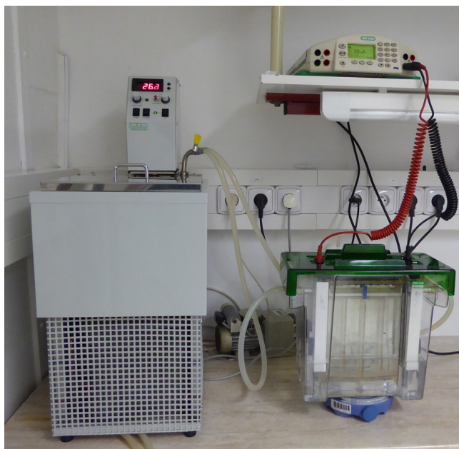
Figure 1. The setup of the electrophoretic apparatus (lower right corner) with cooling thermostat (left) and power supply (upper right corner)
