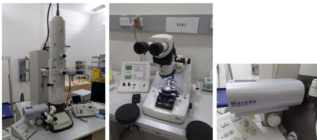
Figure 3. JEM-1011 electron microscope (left), Leica EM UC6 Ultramicrotome (middle), Morada CCD camera (right)
