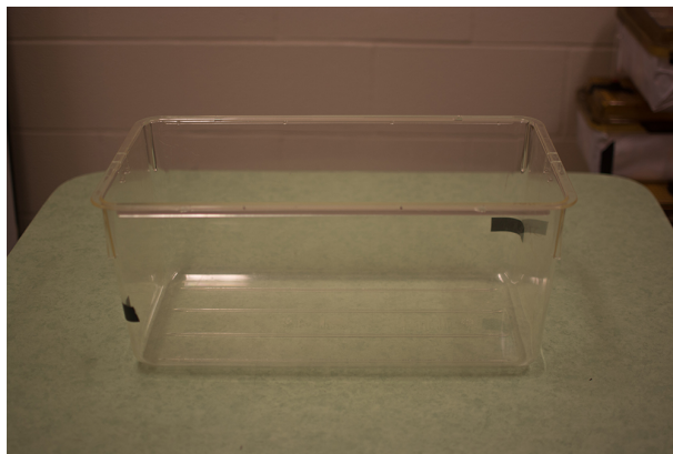
Figure 1. Adaptable apparatus. Photograph of an acrylic glass cage (50 cm x 25 cm x 20 cm) used for Procedures A-D.
