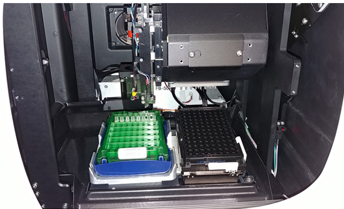
Figure 8. Arrangement of sensor tray and sample tray in Octet RED96. The sensor tray is placed on the left while the sample tray on the right. Close the door of the Octet RED96 machine.
