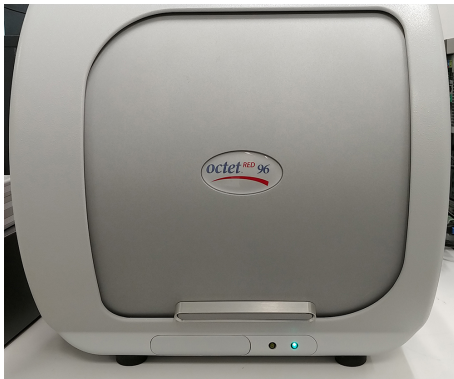
Figure 1. Octet RED96 machine. Switch power on to warm up Octet RED96 machine. When the blue indicator light is illuminated as shown, the equipment is ready for use.
