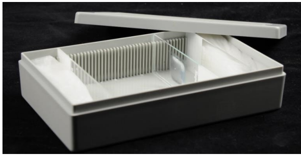
Figure 1. Humid chamber made from a slide box, in which slides can be stored in the fridge and also used as an incubation chamber for pollen germination and tube growth
