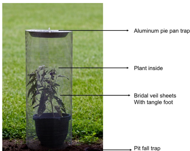
Figure 7. Final trap setup. Final trap integrates the three bridal veil sticky traps, Aluminum-pie pan trap, and two pitfall traps to examine and quantify the insect diversity associated with the host plant inside the cage.
