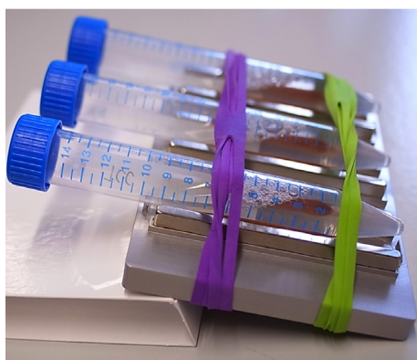
Figure 9. Recovery of tethered circularization products. Tubes containing the ligation products are mounted on a DynaMag-96 Side Skirted Magnetic Particle Concentrator. The beads are reclaimed, and the supernatant is discarded while the tubes are placed in the magnet.
