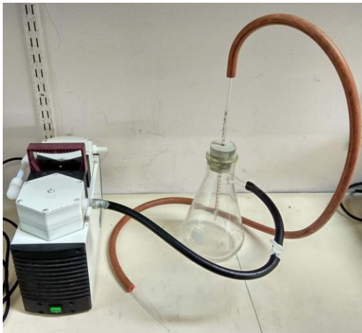
Figure 6. Filter flask connected to vacuum pump
