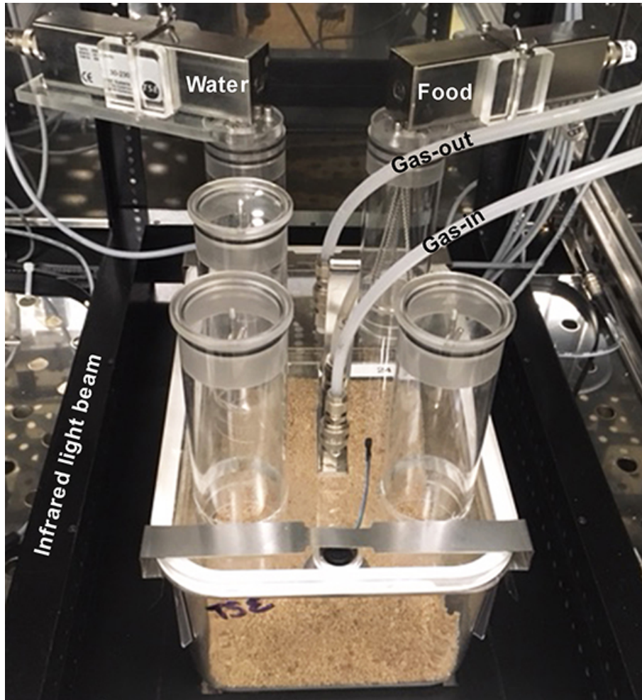
Figure 2. A mouse housing box for the PhenoMaster TSE system. Each box is equipped with tubing for gas in and out, weight sensors for water and food, and an infrared light beam frame for locomotor activity.
