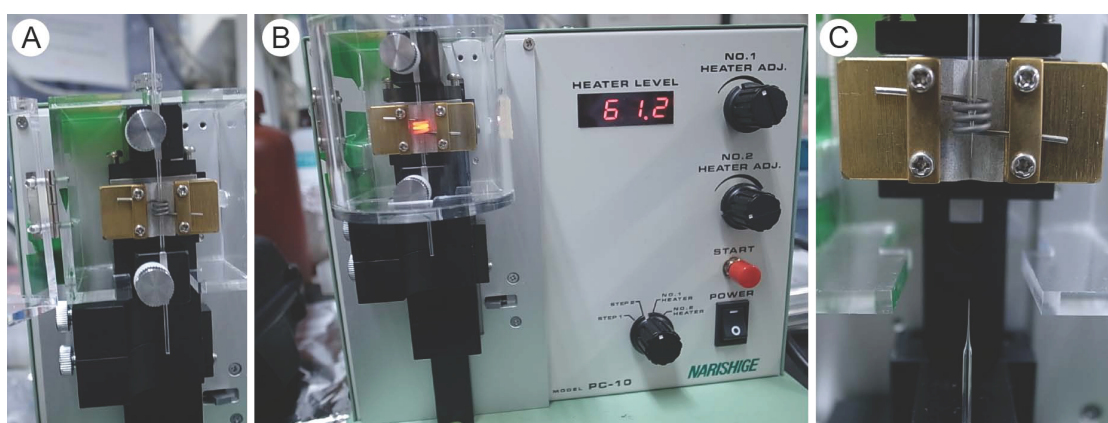
Figure 3. Preparation of glass capillaries by the puller PC-10. Fixation (A), heating and extension (B) of a glass capillary on PC-10. A glass capillary with sharp tip end (C).
