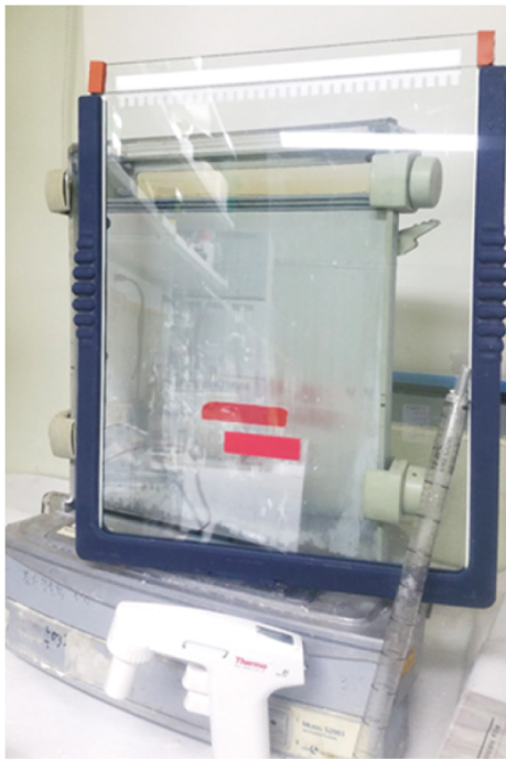
Figure 2. A picture of assembled gel in the gel-casting chamber with the automatic pipette aid
