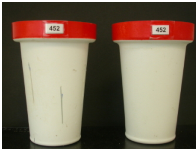
Figure 3. Pots used in PHENOPSIS experiments. Inner pots (left) have extended holes for enhanced soil drying (visible as two lines on the surface of the pot). Holes are nearly identical in all inner pots, thus differences in soil drying dynamics are minimal. Outer pots (right) are not perforated. Source: http://bioweb.supagro.inra.fr/phenopsis/ .
