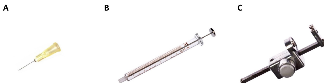
Figure 1. Components to assemble a Hamilton repeating dispenser: hypodermic needle (A), Hamilton syringe (B), and repeating dispenser (C)
