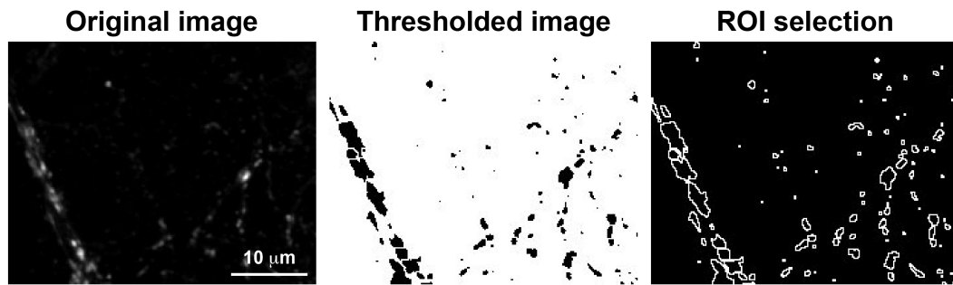
Figure 7. Example of the threshold based selection of FM1-43 labeled ROIs. Image on the right depicts outlined ROIs determined based on the threshold and particle size.
