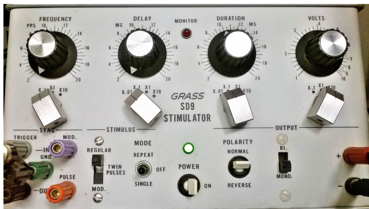
Figure 4. Grass instruments SD9 stimulus isolator settings. Frequency–0, Delay–0, duration–10 x 0.1, Volts–7 x 10, output–mono, polarity–normal.
