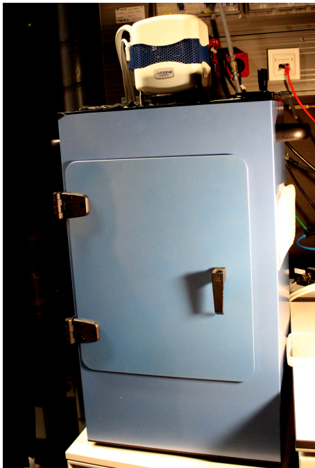
Figure 3. Dark box with a Photometric Evolve EMCCD camera
