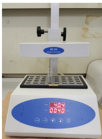
Figure 2. Evaporation of sample at 40 °C under a stream of nitrogen using sample concentrator (MD200-2). The spray nozzle was inserted into a glass tube which was placed to aluminum dry bath heating block. Sample was dried at 40 °C under nitrogen gas.
