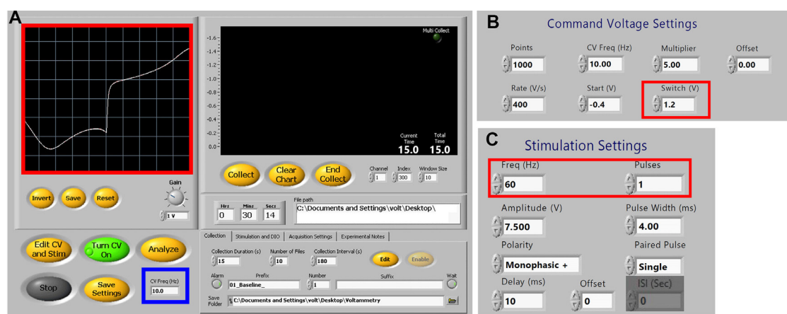
Figure 4. Demon Voltammetry setup for dopamine detection. A. User Interface showing typical experimental settings with ideal current-voltage plot from an electrode (red box). For carbon fiber electrode conditioning, the CV freq (blue box) may be increased from 10 Hz to 60 Hz. B. Command Voltage settings. Switching potential can be adjusted as needed (red box; see Note 4). C. Stimulation settings for single pulse experiments (frequency is not used for single pulses). Frequency and pulse number (red box) can be adjusted as needed for multipulse experiments (see Note 5).
