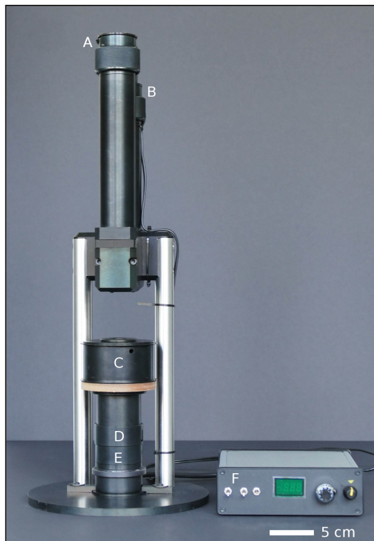
Figure 1. A double-beam photometer used for measurements of transmittance changes resulting from blue light-activated chloroplast movements. Key components: A. blue LED housing; B. red LED housing; C. measuring chamber; D. 660 nm interference filter; E. receiver photodiode; F. electronic controller.
