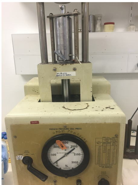
Figure 1. Cell lysis using a French press. Photo of a French Pressure Cell that can efficiently lyse microalgae cells, including diatoms. Algae cell extracts in ice cold buffer are placed in the ice-cold stainless steel French Pressure Cell and hydraulic pressure applied. Once at 140 MPa the outlet to the Cell is slowly opened. The cells lyse as they emerge from high to ambient pressure and the cell extract is collected into a 15 ml or 50 ml polypropylene tubes. A slow flow rate of sample out of the Cell ( \sim 1 to 2 \text{ drops sec}^{-1} ) is maintained to ensure the pressure is maintained (see Video 1, acknowledgement Bratati Mukherjee).
