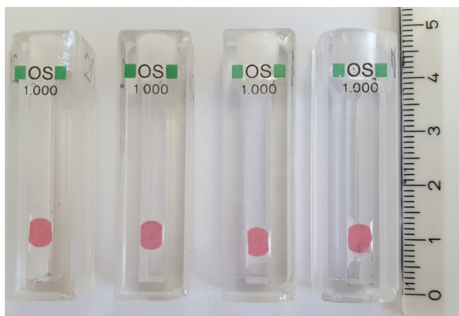
Figure 1. Oxygen monitoring cuvettes. The total volume per cuvette is 1.4 ml. A PreSens oxygen sensor spot (red) was cut and glued in place as described above.
