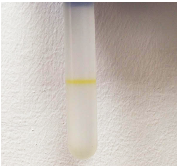
Figure 3. OMVs (the yellow line within the tube) are suspended within one of the fractions of the density gradient, after ultracentrifugation at approx. 246,000 x g for 6 h
