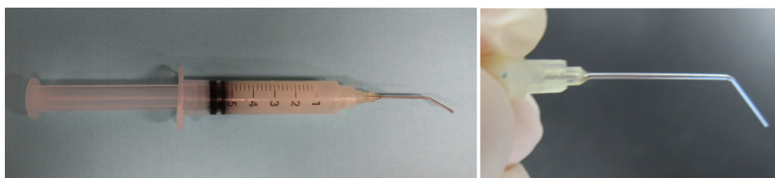
Figure 2. Petroleum jelly filled syringe used for preparing the extracellular stimulation/recording wells
