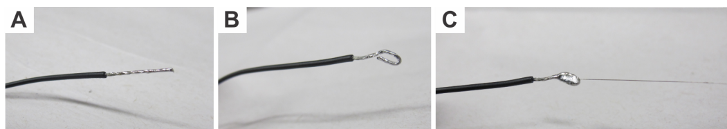
Figure 3. Preparation of extracellular stimulation/recording electrode. A. Electrical wire with insulated and tin-solder coated front part; B. Same wire, bent into a loop; C. Stainless steel wire attached to loop with tin-solder.
