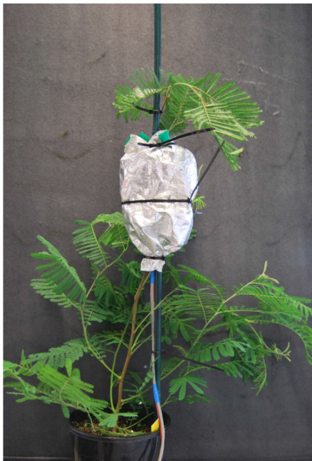
Figure 7. Completed insulation of the external sapflow gauge. Gauges installed on a small branch of a potted Acacia mearnsii were insulated with polystyrene and covered in reflective foil.
