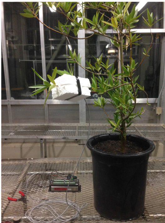
Figure 1. Miniature external sapflow gauge with 10 m lead cable connected to a small branch of a potted Umbellularia californica plant and a Campbell Scientific CR10X data logger
