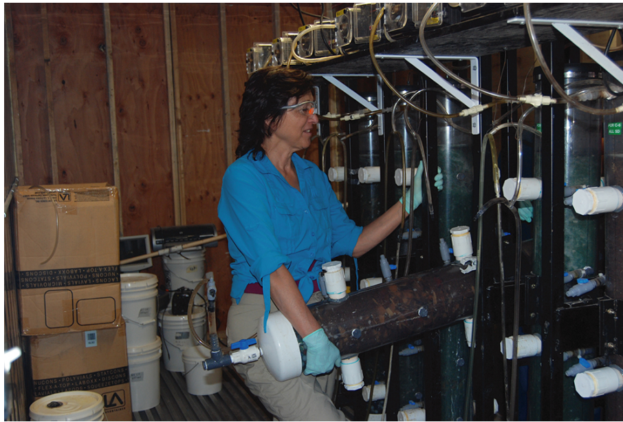
Figure 6. Intact columns and supporting hardware in use during sampling process. One of the columns is being tilted horizontally for sample bag retrieval to enable analysis during the experiment.
