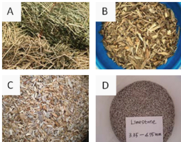
Figure 2. Examples of solid-phase matrix components deployed within columns. A. Alfalfa hay; B. Woodchips; C. Sawdust; and D. Limestone. Alternative substrates such as sand or other organic solid-phase materials could have relevance to alternative applications such as studying subsurface flow or aquifer recharge.
