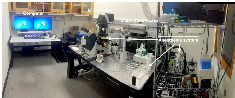
Figure 1. Inverted Multi-photon setup. The imaging setup includes an inverted confocal microscope with 25x water objective fitted with a culture dish holder, multi-photon laser and computer.
