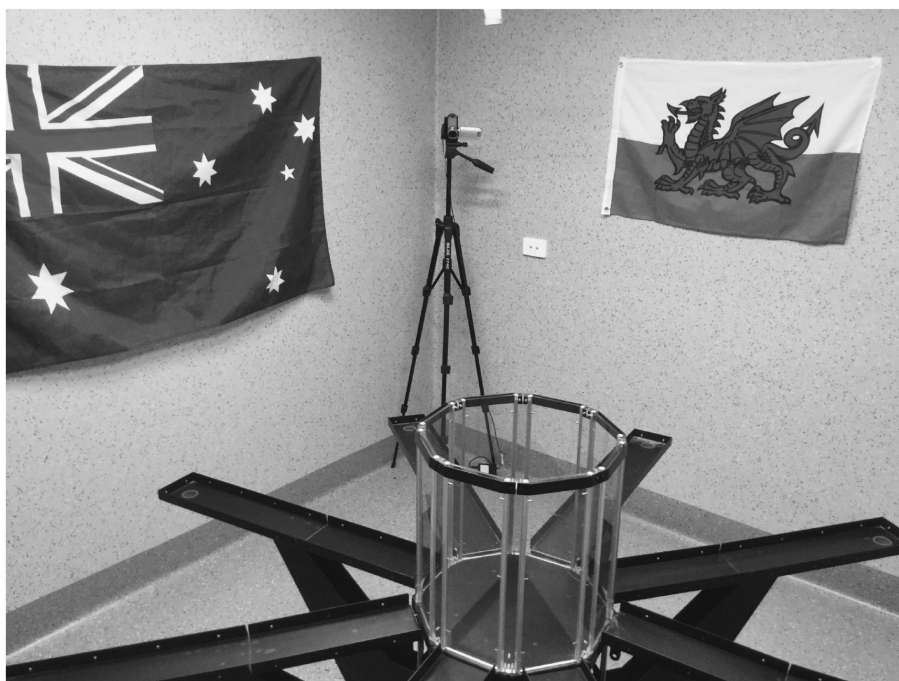
Figure 1. Radial Arm Maze (Lafayette Instrument Company) with automated Perspex doors and spatial cues placed around the maze. The camcorder is placed on the tripod facing downwards (approximately 45° to the maze). The camcorder can also be attached to the ceiling directly above the maze.
