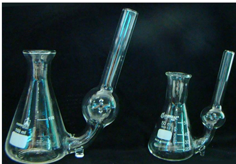
Figure 1. Adapted Erlenmeyer flasks (100 and 50 ml) used in SCV analyses. For an adapted Erlenmeyer flask of 100 ml capacity, we used 25 ml of culture medium and 500 mg of fresh cells. For an adapted Erlenmeyer flask with 50 ml capacity, we used 10 ml of culture medium and 200 mg of fresh cells, with a ratio of 20 mg fresh cells to 1 ml of culture medium.
