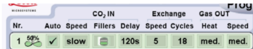
Figure 3. Settings used for critical point drying using the Leica EM CPD300
