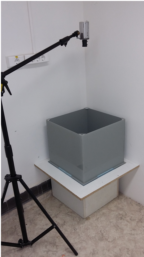
Figure 1. Custom-made OF box prepared from common household plexiglass. Digital video tracking can be performed with a conventional coloured CCD camera fixed and positioned above the OF arena with a telescopic tripod stand.
