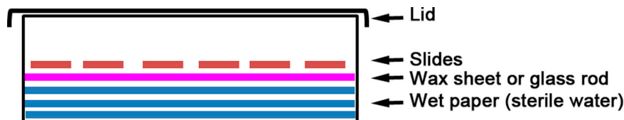
Figure 1. Wet chamber. The principle of the wet chamber is to keep the sample moist at all times.
