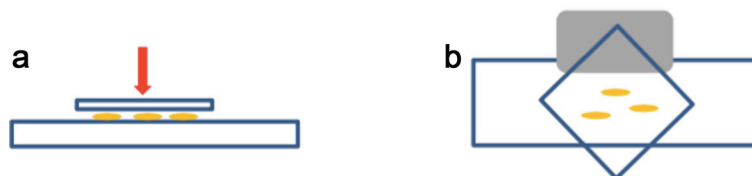
Figure 3. Squash method. For squashing, enzymatically digested root tips are placed between a microscope slide and a coverslip (a). The coverslip is placed as shown in (b) to be removed easily by using the edge of a razor blade (grey shape) under one side of the coverslip after freezing in liquid nitrogen.
