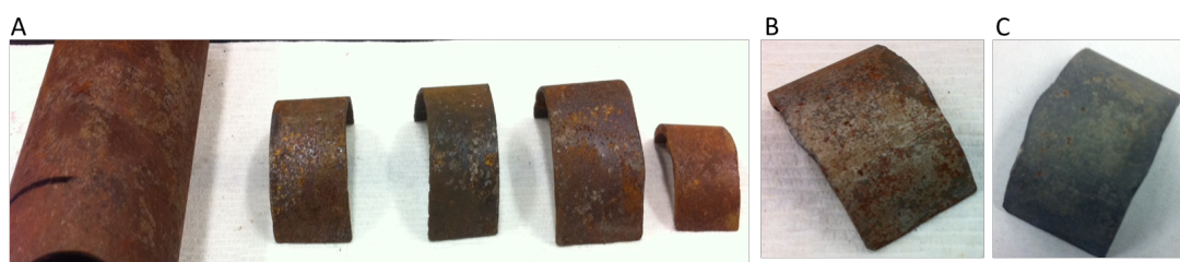
Figure 2. Visual examples of metal samples treated with rust removal agents. Metal samples before treatment (A), after 2 h of treatment with a commercial rust removal agent (B; Rust-Oleum) and after thirty minutes treatment with 10% oxalic acid (C).
