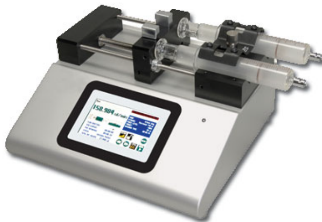
Figure 2. KDS Legato™ 200 syringe pump (modified picture from http://www.kdscientific.com/products/pumps/Legato200.asp )
