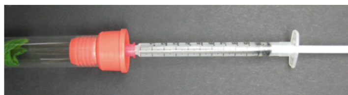
Figure 3. Gas sampling from a glass tube capped with a septa stopper
