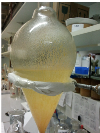
Figure 1. Typical set up for liquid-liquid partition using a separating funnel
