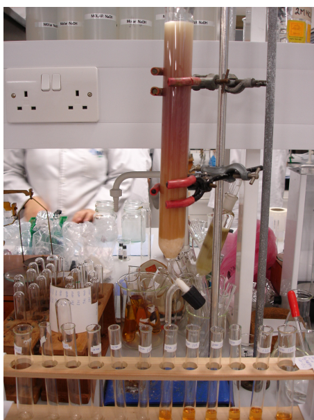
Figure 4. Typical set up for column chromatography
