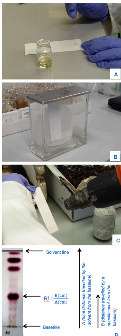
Figure 3. Thin layer chromatography (TLC) analysis. A. Spotting of sample on TLC plate; B. Spotted plate placed in the TLC tank for elution; C. Heating of plate; D. Calculation of Rf values for triterpene (pink) spots.
