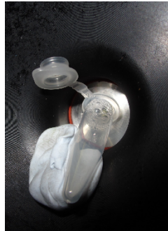
Figure 2. An example of xylem sap being collected from a sample enclosed in a Scholander pressure chamber. The collection tube can be held in place with Blu-Tack or modeller's clay.
