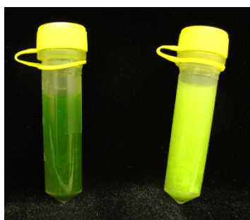
Figure 7. An example of the homogenization obtained after the use of cell lysis machine and stainless steel bead on the leaflet and green seed samples shown in Figure 4. Note that this method is only effective for soft, herbaceous leaves or green seeds.
