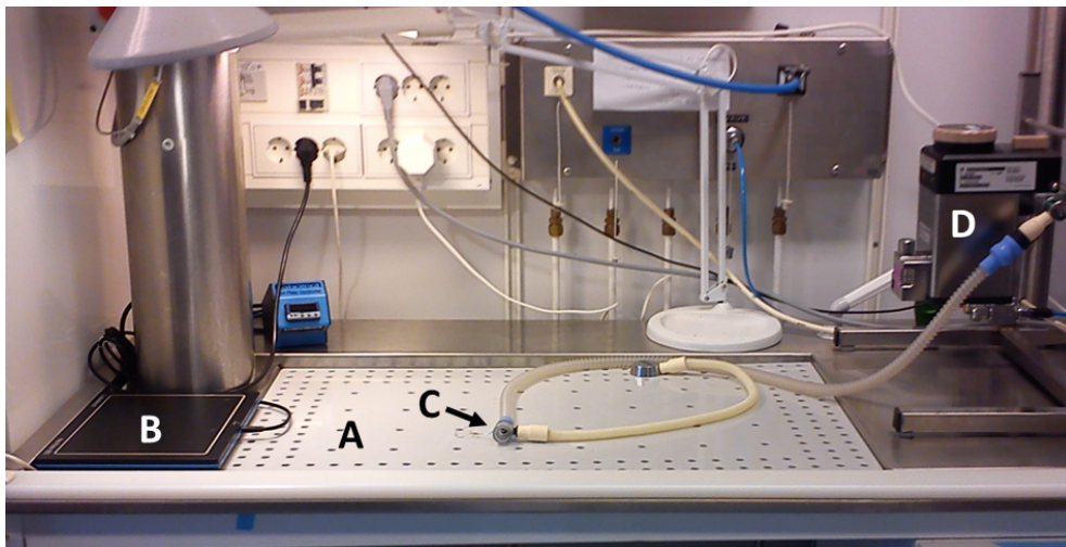
Figure 4. Ventilated area for surgery (A). Heating plate for keeping pups warm (left, B), nasal mask for anesthesia (center, C) and anesthetic vaporizer (right, D).
