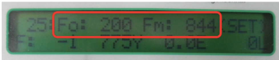
Figure 5. A photo of the display when setting Fo and Fm ("Mode" menu 25)
