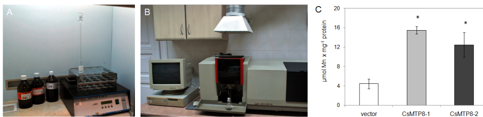
Figure 5. Details of the analysis of Mn accumulation in Arabidopsis plants. A. Dried plants were digested in closed glass vessels by heating in 10 ml of 65% HNO 3 in heating digester at 150 for 12 h. B. Atomic absorption spectrophotometer was used to estimate Mn content in the solution following digestion (mineralization). C. The example data are present as means ± standard deviations of three independent experiments with at least 15 plants each. Asterisks indicate significant differences between the line transformed with empty vector and two lines carrying CsMTP8 (b) (P<0.05; ANOVA Student-t tests).
