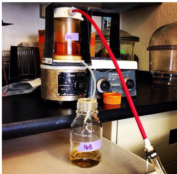
Figure 1. Amicon ultrafiltration setup. The ultrafiltration cells are connected to compressed nitrogen gas. The gas applies pressure, forcing the supernatant through the 100 kDa filter membrane. Vesicles stay in the concentrated supernatant while smaller proteins and liquid supernatant flow into waste container.
