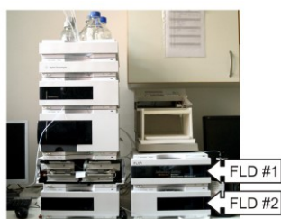
Figure 1. The Agilent 1200 HPLC system equipped with an autosampler and two fluorescence detectors marked as FLD #1 and FLD #2
