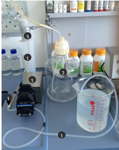
Figure 2. Assembly of filter sterilization for large volumes of artificial urine. The same procedure is applicable for pooled human urine. Relevant visible parts are marked according to equipment list.
