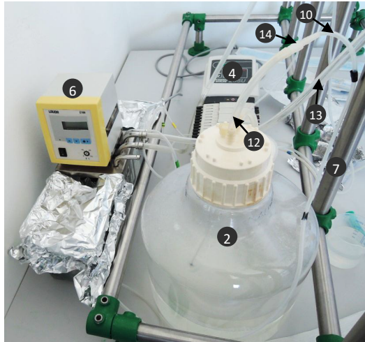
Figure 3. Connection of water cycle and urine supply. Water bath is directly connected to the bladder models (not shown), the urine is pumped from the reservoir using a peristaltic pump (use a channel for each model). Relevant visible parts are marked according to equipment list.
