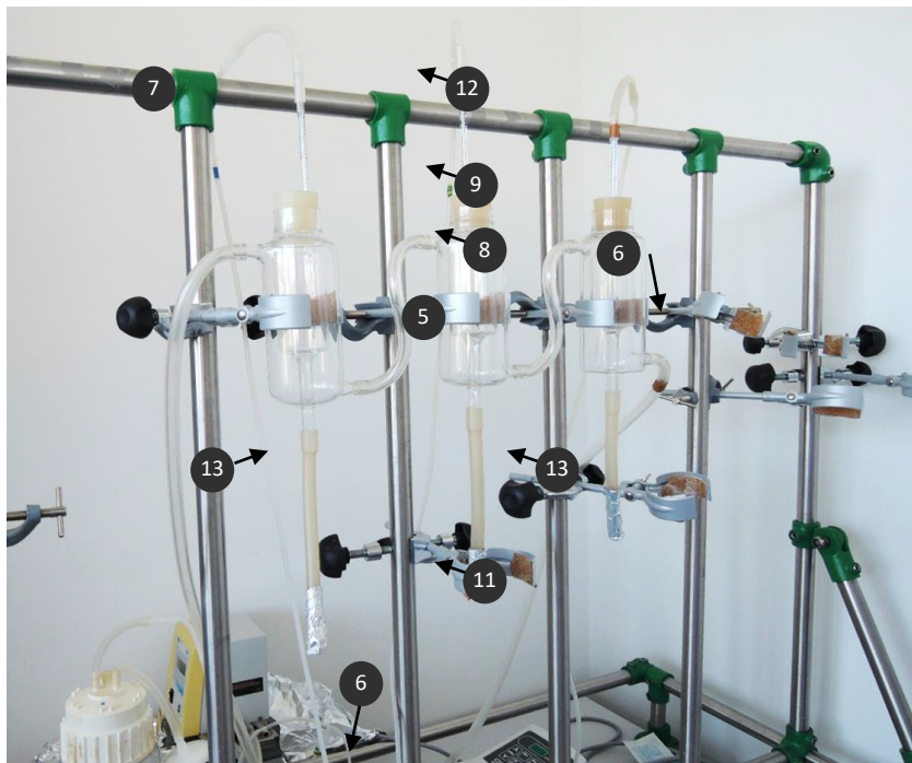
Figure 4. Bladder model system with three bladders after connection of tubings prior to catheter insertion. Relevant visible parts are marked according to equipment list.
