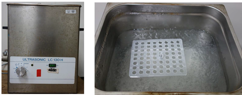
Figure 4. The dissolution of protein with ultrasonic vibration. Left panel is the ultrasonic machine. Right panel shows the protein sample is resuspending in the cold bath with ultrasonication.
